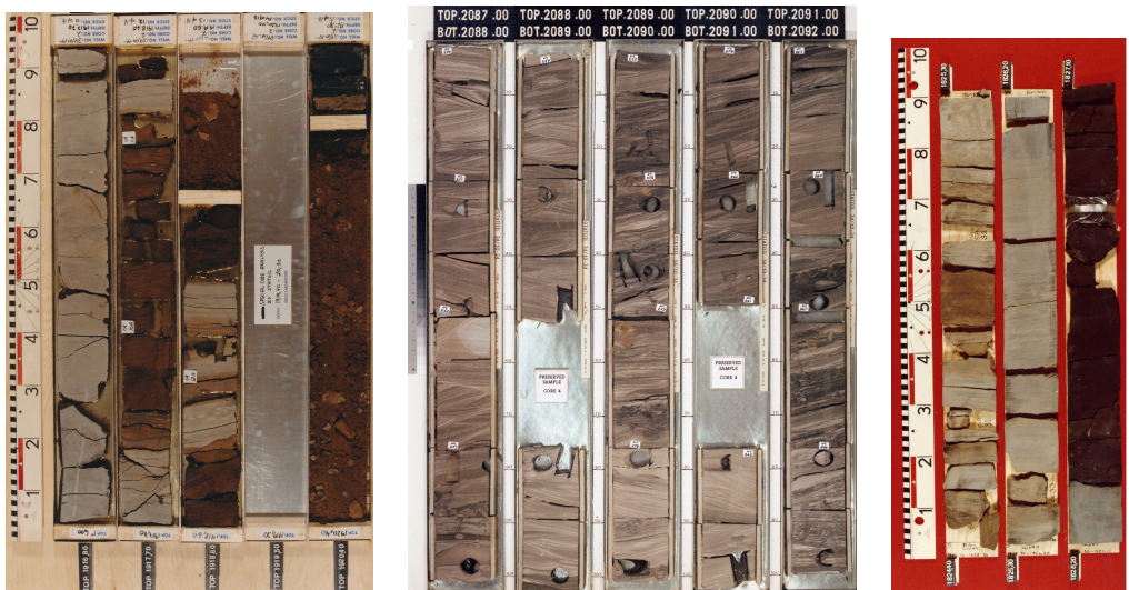
Figure 3.2.2. Left: Upper Ness (N-3), well 34/10-14 at 1916-1921m, north-middle part of Gullfaks. Possible soil profile with coal beds. Middle: N-2, well 34/10-34 at 2087-2092m, Gullfaks west. Heterolithic, bayfill sandstone with small-scale hummocky stratification. Right: Lower Ness (N-1), well 34/10-1 at 1824-1827m, southern Gullfaks. Shows a crevasse spilled over a thick coal-mash layer. From NPD-Factpages (2015).
