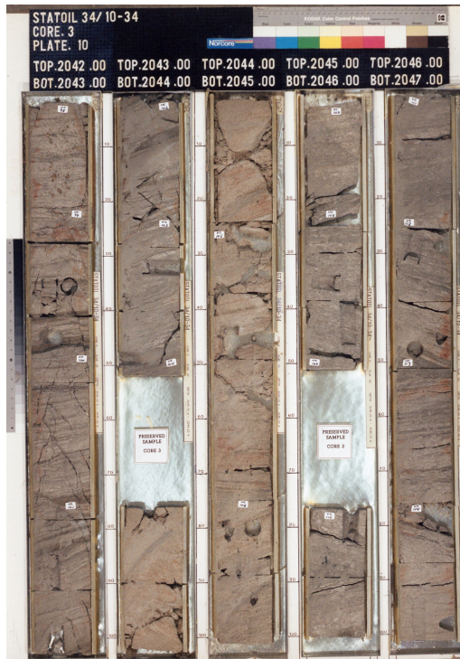
Figure 3.2.4. Lower Tarbert formation at well 34/10-34, depth 2042-2047m. Bioturbated, planar to low-angle laminated sandstone. From NPD-Factpages (2015).
