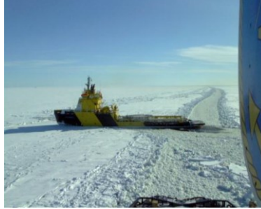
Figure 2.4: Brash ice channel – made by an icebreaker (Riska 2013)
