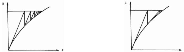
Figure 7.9: No updating of \mathbf{K}_I (left) and \mathbf{K}_I updated after 1. iteration (right) (Moan 2003)
