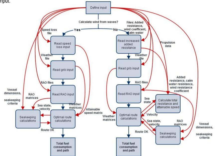
The functions in the program is divided into read functions and calculate function. ShipX is used to create input files for the program. ShipX calculates the added resistance operator and the transfer functions for the vessel. The running time of the program is high for actual wind, but acceptable for estimated wind
