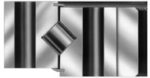
Figure 4: Cross row roller ring[1]
