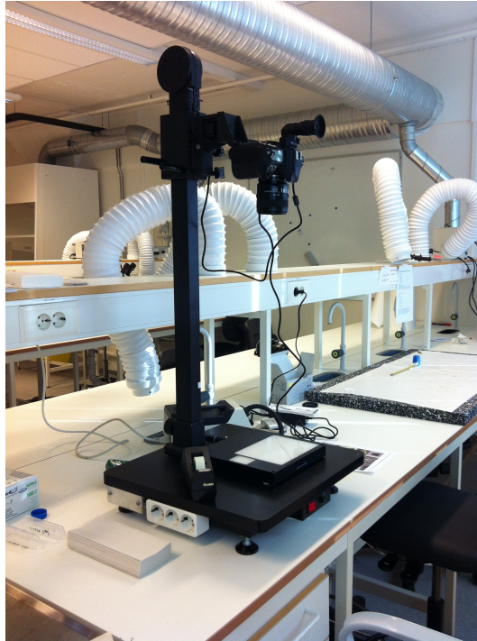
Figure 2-6 – The rig used to stabilize the camera when taking close up images of the bryozoan colonies
