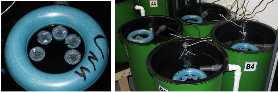
FIGURE 1: Picture form experiment tanks. Left ; the five cell strainers with a parafim on top floating on the water surface restricted by the floating ring (20 cm diameter). Right ; four of the experiment tanks with cell strainers and floating rings placed on the water surface.
