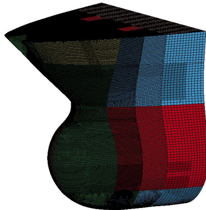
Figure 6.12: Bow model used in the collision analyses.
