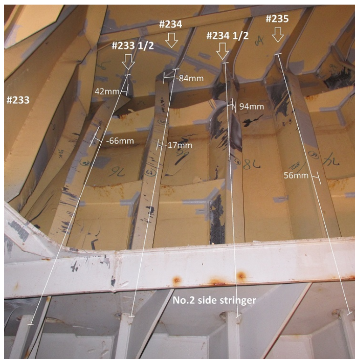
Figure 3.9: Deformation of plates and frames #233 - #235, [5]
