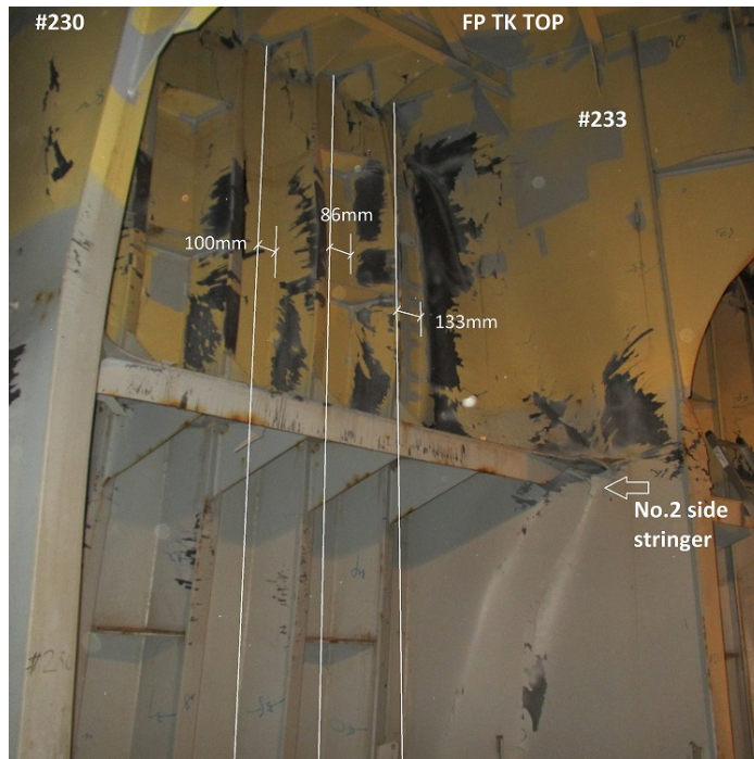
Figure 3.8: Deformation of plates and frames #230 - #233, [5]
