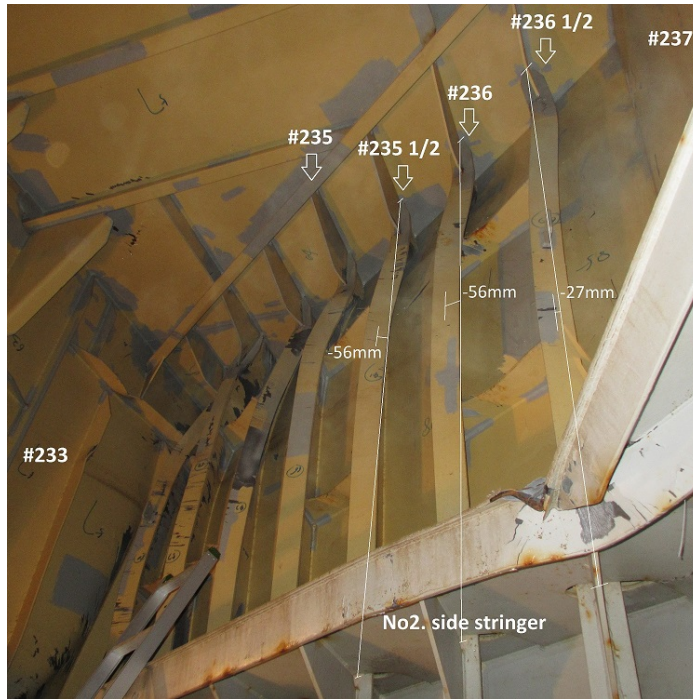
Figure 3.11: Deformation of plates and frames #233 - #237, [5]
