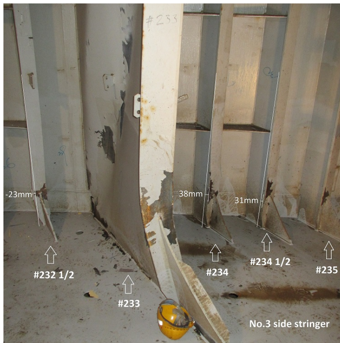
Figure 3.12: Deformation of plates and frames #232 1/2 - #235, [5]
