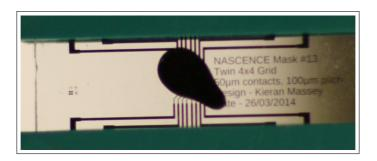
Figure 3.2: A photograph of the SWCNT material on its glass slide.
