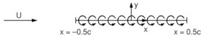
Figure 4: 2D linearized body boundary condition for a flat plate in steady infinite flow (Faltinsen 2005).
