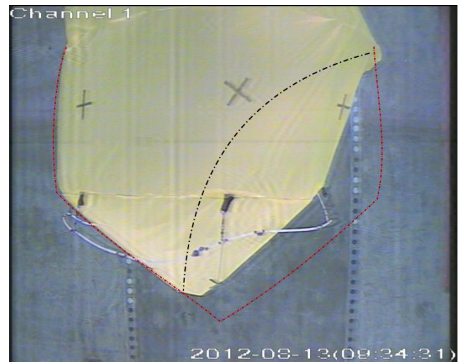
(b) Deformation pattern for 70% filled cylindrical bag, for V_c > 0.3 m/s. Undeformed borders for 100% full bag at 0 m/s indicated in red. The hemispherical cup deformation is indicated with a dotted black line.
