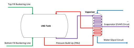
Fig. 1. Schematic of the LNG tank and Vaporizer system on KV Bergen and MF Korsfjord
