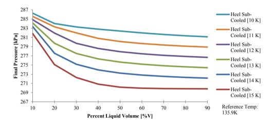
Fig. 3. Final Tank Pressure After Complete Liquid and Vapor Mixing Given Different Initial Liquid Temperatures
