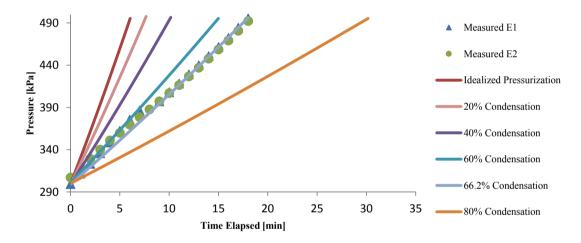
Fig. 7. LNG Tank Pressurization Time with Vapor Condensation
