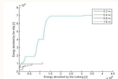
In the results shown above the energy absorbed by the ship without ice strengthening are in the vertical axis, and the energy absorbed by the iceberg in the horizontal axis. The different radius in front of the iceberg are shown with the different color lines. As seen in the figure above the largest iceberg give the stepes curve meaning that more percentage of the total energy goes to deform the shipside. The same tendency is seen for the two other ships.
