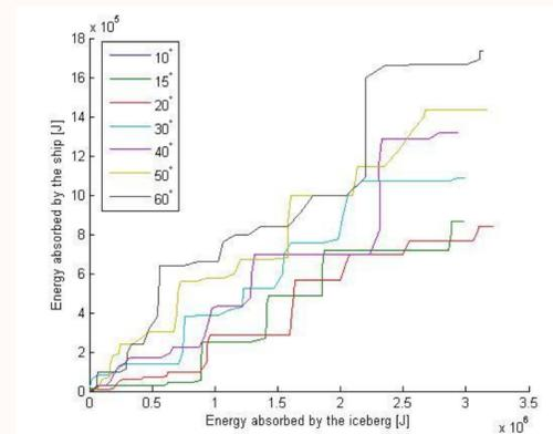
The figure above present the second largest iceberg on the ship without ice strengthening, with different angels of the cone. The damage to the ship is increasing with the angle of the cone. As the forces are about the same.
