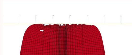
The figure above present the largest deformation of the ship without ice strengthening, which are about 5cm and barely visible on the figure. The iceberg has deformed to the side due to the Poissons effect. This may be unrealistically high deformation of ice since ice is known to be quite brittle.
