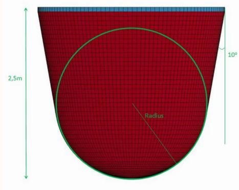
The values chosen for the iceberg is as shown the figure above, and the radius is varied. The effect of confinement is also considered with change of the cones angle.
