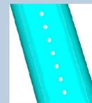
As a potential collapse mechanism, the buckling strength of the shell needs to be investigated further than the method used in the preliminary design process. To reduce computational time and simplifying the modelling process, the sections between ring stiffeners are chosen for the analyzes.
