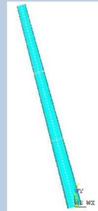
Due to the large wind pressure acting on the structure, it is beneficial with cut-outs, acting as ventilation for the flare tower. The alignment and positions of the cut-outs can also be used to prevent or limit vortex induced vibrations, which will be a topic of discussion later in the thesis. These cut-outs have a diameter of 0,3 meters, with an elevation of 1 meter between each cut-out. Each section counts four cut-outs with an angle of 90 degrees between each cut-out.
