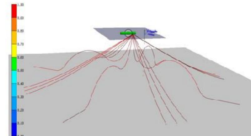
In a coupled analysis are the vessel motion and the mooring line and riser dynamics calculated simultaneously. The interaction effects are then taken into account, and accurate floater motions and slender structure dynamic loads are obtained. The main disadvantage with the use of a coupled approach is that the analyses are time consuming and require a large amount of CPU time. (Ormberg et al., 1997, Ormberg and Larsen, 1998, Heurtier et al., 2001, Gurusurthy et al., 2011)
