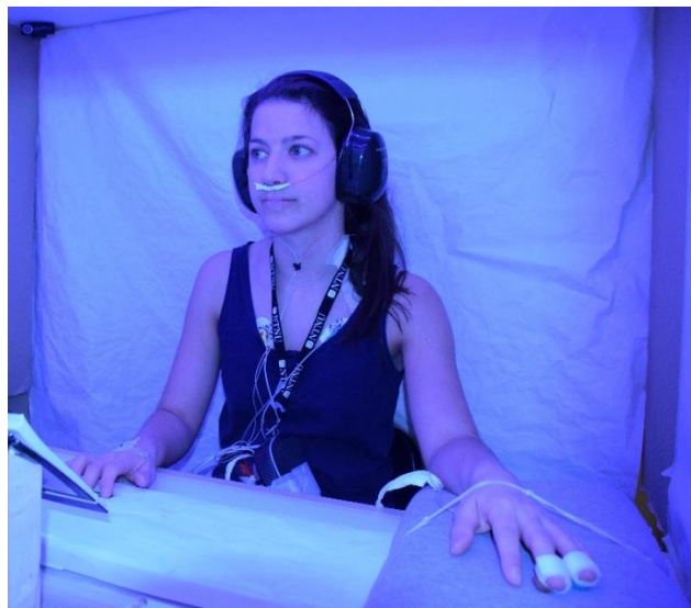
Figure 2. Sensors; GSR (left hand), ECG (chest), airflow (nostrils), thermometer (neck) and accelerometer (right hand)
