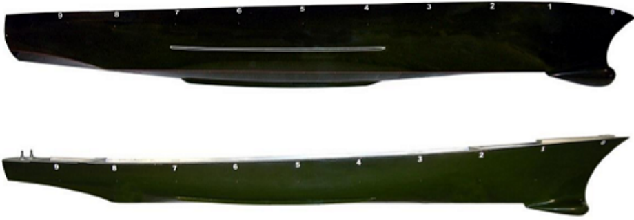
Figure 20: DTMB 5512 ship model. Bilge keels shown in top image.
