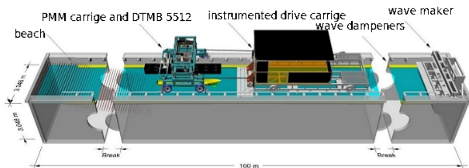
Figure 18: IIHR towing tank
