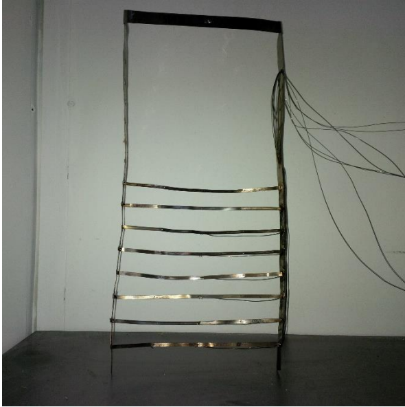
Figure 12: The "thermocouple-ladder" with horizontal steps where the TCs are mounted. The steps are at every two centimetres.
