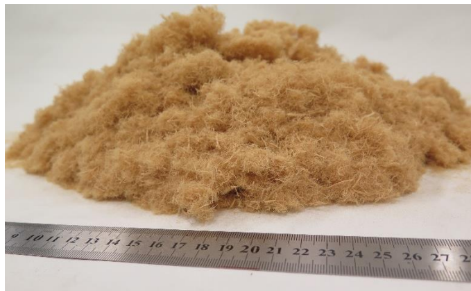
Figure 7: Material V after mixing. The picture shows approximately 60 grams of the material.
