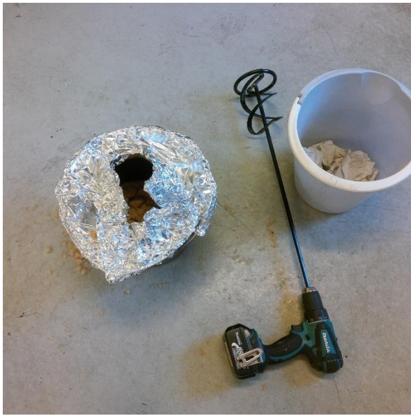
Figure 16 : The equipment used for mixing the insulation with air: A power drill with a paint mixer and a flat-bottomed bucket.
