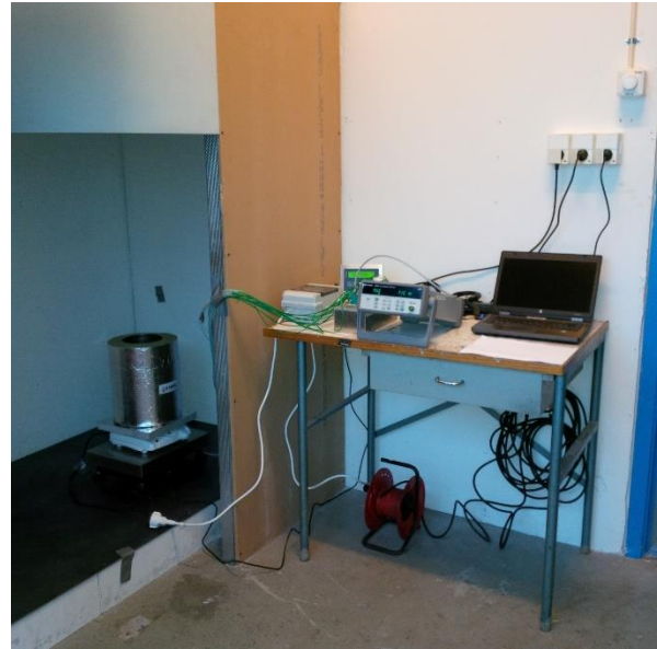
Figure 11: Test setup placed under the extractor hood. On the table to the right the thermostat and the equipment for data logging is placed.
