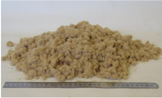
Figure 5: Material T after mixing. The picture shows approximately 80 grams of the material.
