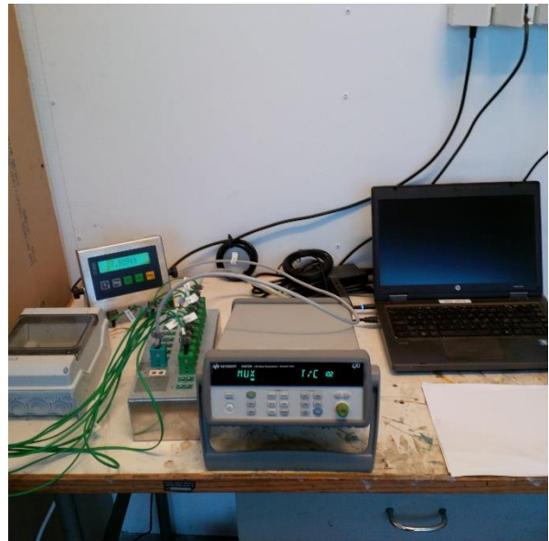
Figure 15: The thermostat and logging equipment: Thermostat, scale display, logger and laptop.
