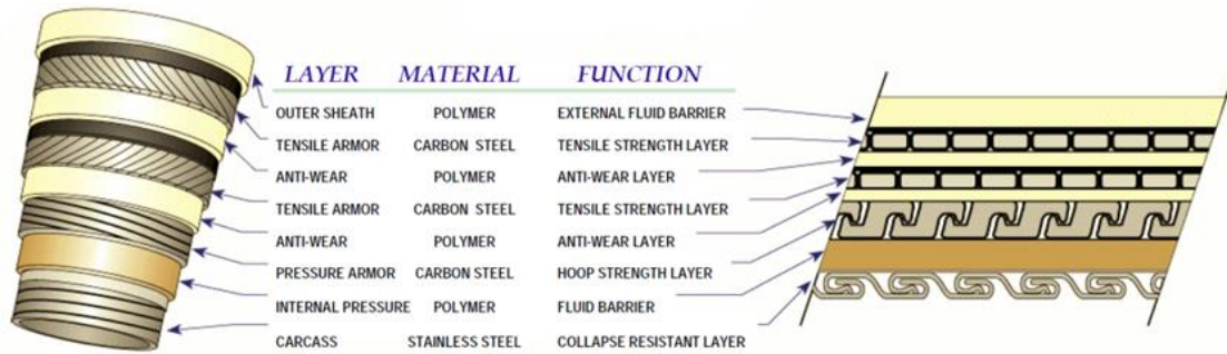
Figure 1-2 Flexible Pipeline Layers
