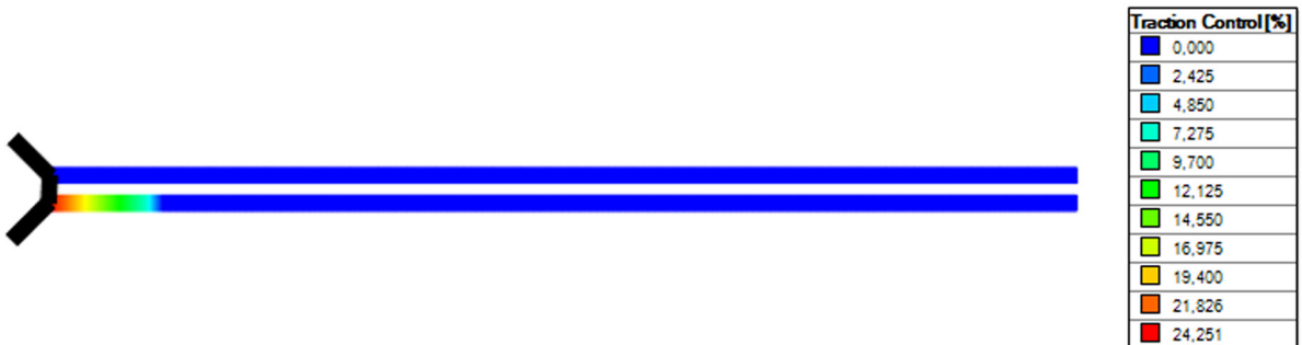
Traction control activity during simulated 0 to 75 meter acceleration event for 4WD vs. RWD concept.
