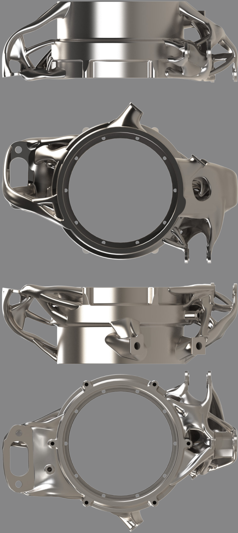
Final 3D model of front upright designed using the topology optimization result as a framework.
