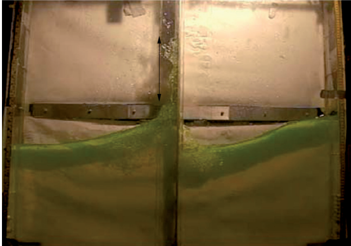
Figure 3-9. The photograph and video recording of the run-up at the screen occurring for 0.9 \leq Sn , h/l = 0.4 , \varepsilon = 0.01 .
