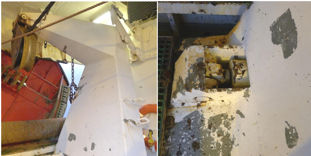
Figure 36 Ice Davits, upper part and socket.
