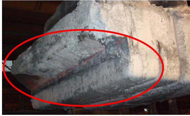
Figure 7: Anode cracked during operation in the electrolysis cell 11 . The picture above shows that a large portion of the bottom left corner of the anode has fallen off due to slot cracks.
