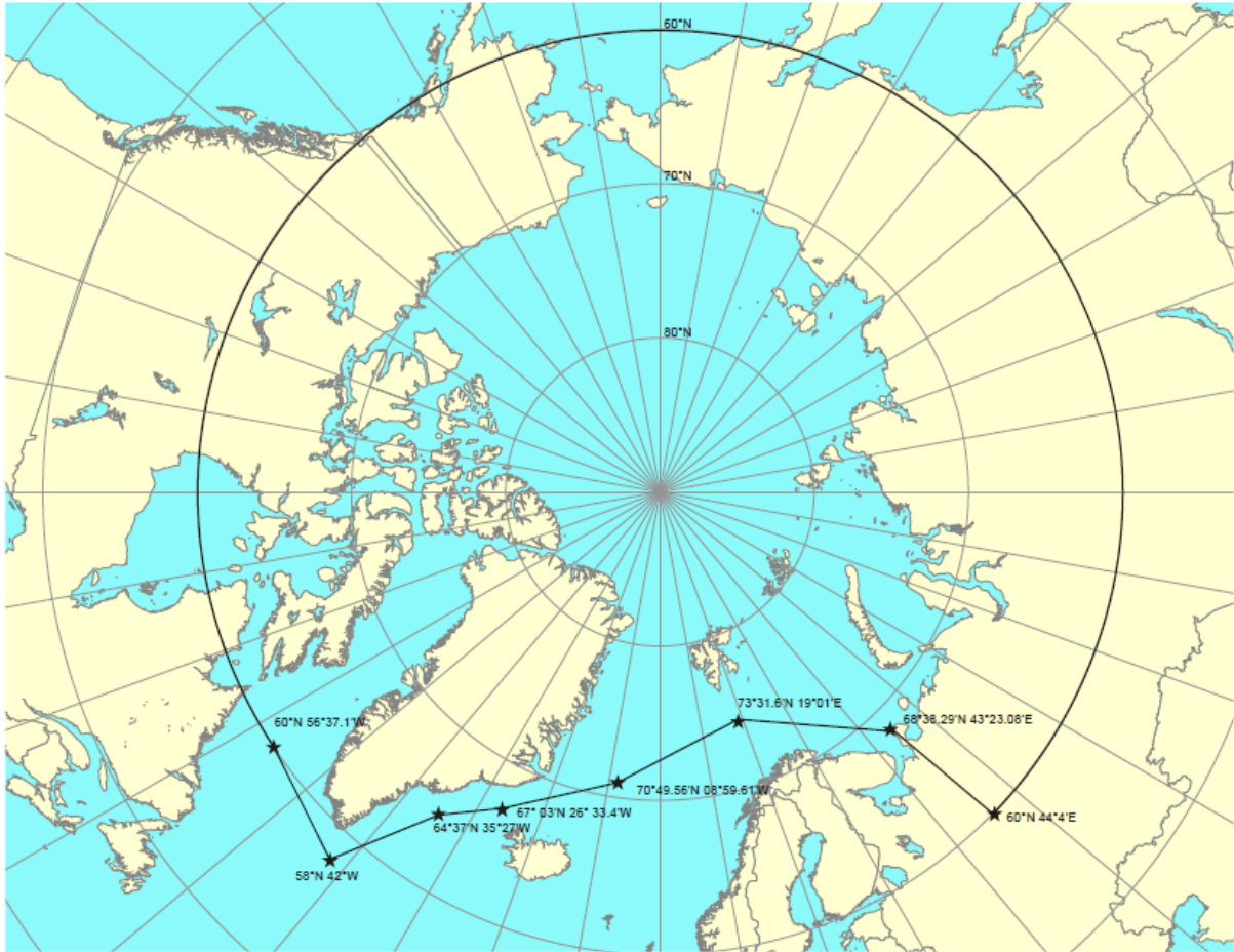
Figure 32 Areas where the Polar Code is to be applicable 10 (26)
