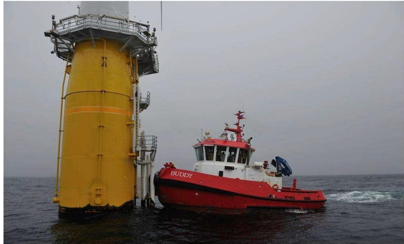
Figure 2.1 - The service vessel "Buddy" in a boarding operation at Hywind. (29)
