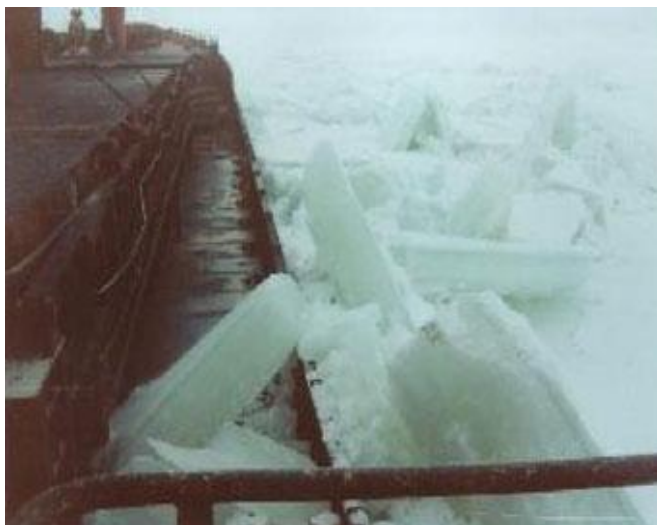
Figure 3-12: Ship in compression ice in the Baltic Sea [24]
