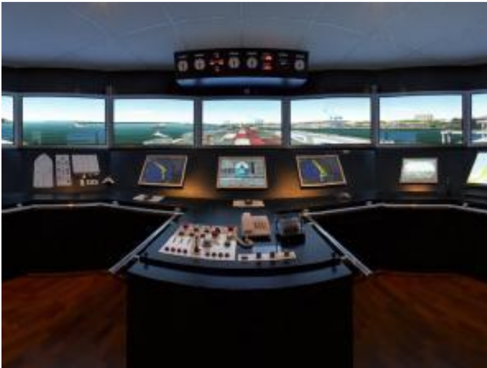
Figure 4.1 Ice bridge simulator, picture of bridge console. picture source; http://www.uniteammarine.com
