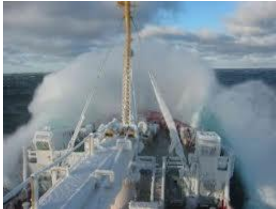
Figure 2.1 Sea splashing made by collision between ship's bow and encountered wave, those icing on rigging can be observed due to wave-generated sea spray. (From Canadian Coast Guard HP, http://www.ccg-gcc.gc.ca )
