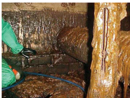
(a) Calcium naphthenate deposit formed inside a coalescer
