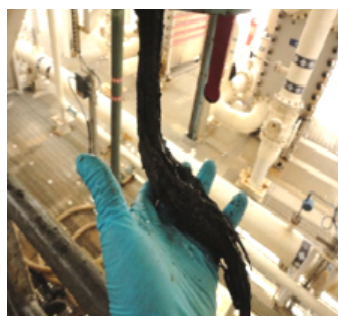
(b) Calcium naphthenate deposit retrieved from a coalescer
