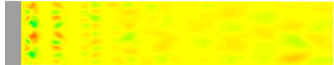
Figure 3.12: Instantaneous plot of streamwise vorticity, \omega_x , plotted in the x - z -plane for grid B4. Re = 300
