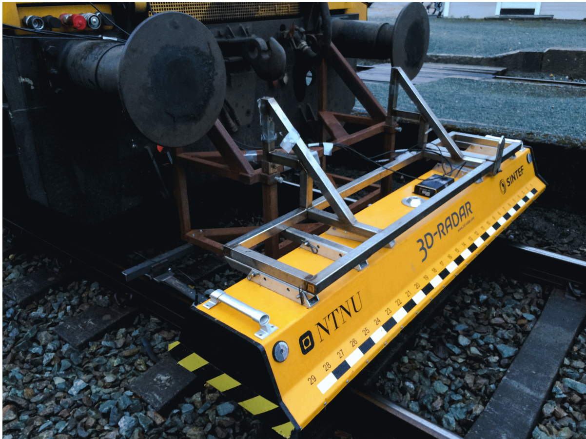
Figure 20: 3d-radar V2429 antenna-array mounted on Robel rail-tractor
