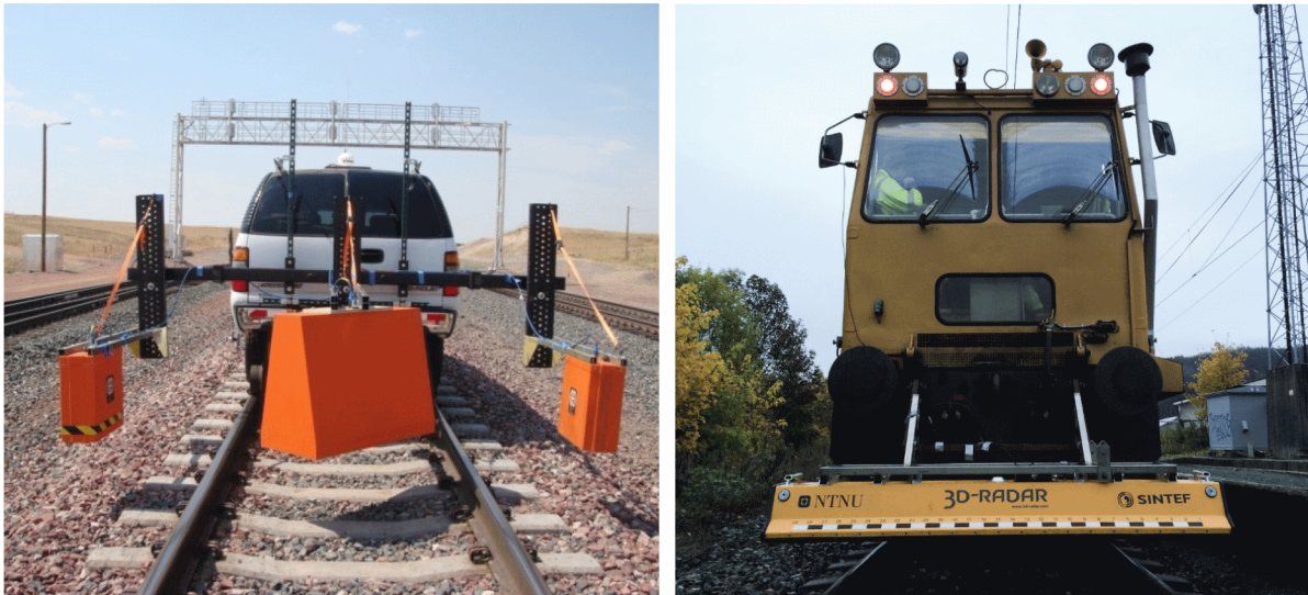
Figure 5: Left: Air-coupled horn-antennas. (Cassidy, 2009) Right: Air-coupled bow-tie antenna array.
