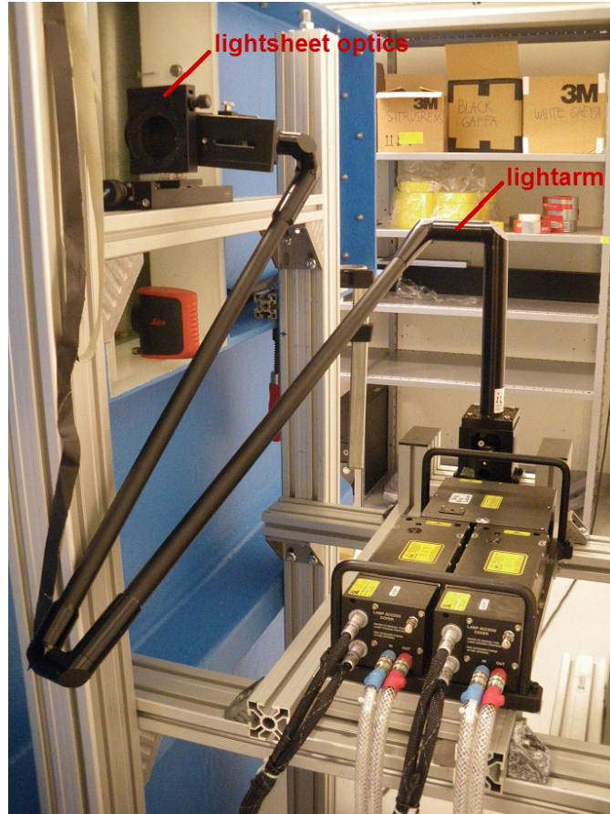
Figure 2.6: The lightsheet optics that transform the laser beam into a lightsheet.
