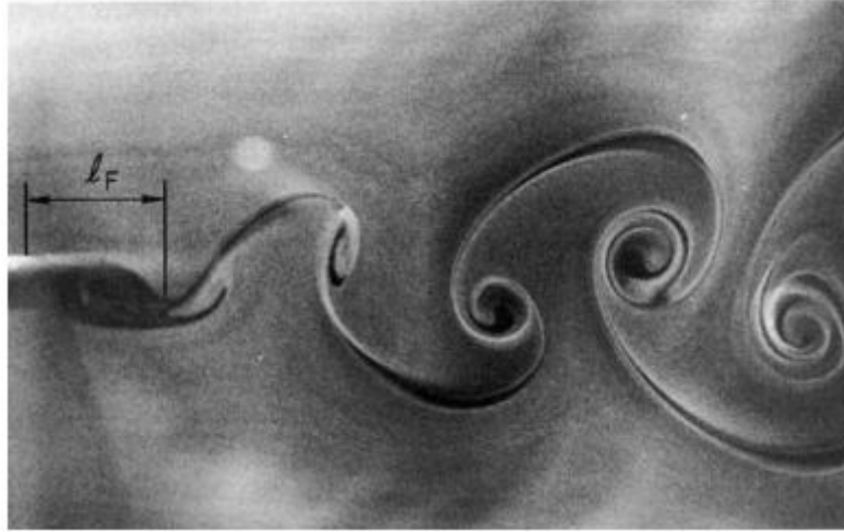
Figure 6.5: Definition of the eddy formation length L_f , as observed from flow visualization in the wind tunnel by Griffin [5].
