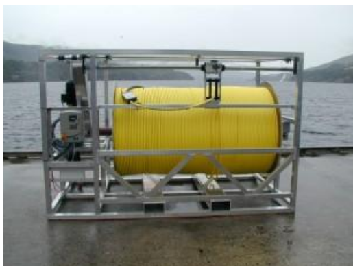
Winch with 2000 m cable
