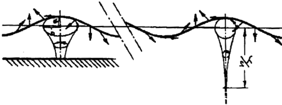
Figure 2-4 Motion of water particles in deep water (left) and shallow water depth (right) [8]
