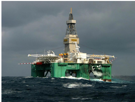
Figure 4.9: A semi-submersible platform, the drillrig “Eirik Raude” owned by Ocean Rig, [28].
