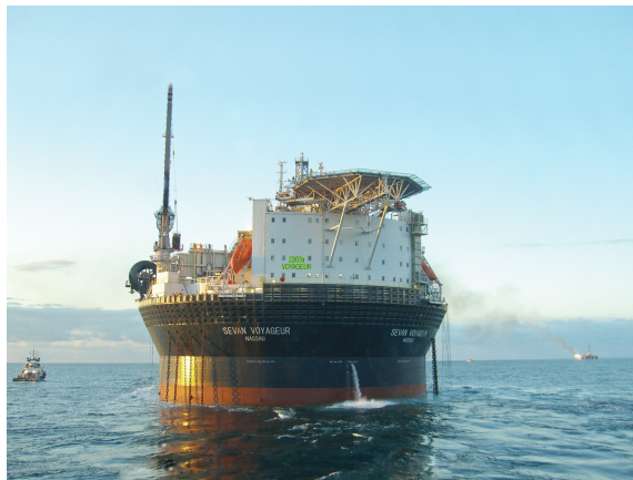
Figure 4.8: Example of circular FPSO, the Sevan Voyageur by Sevan Marine [37].
