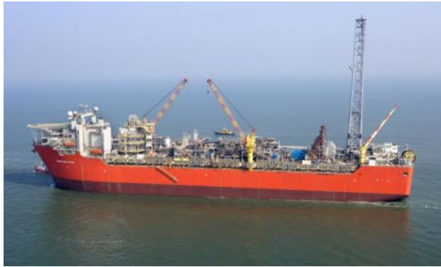
Figure 4.6: Terra Nova FPSO. It utilizes a turret mooring assisted by a DP-system. [11].
