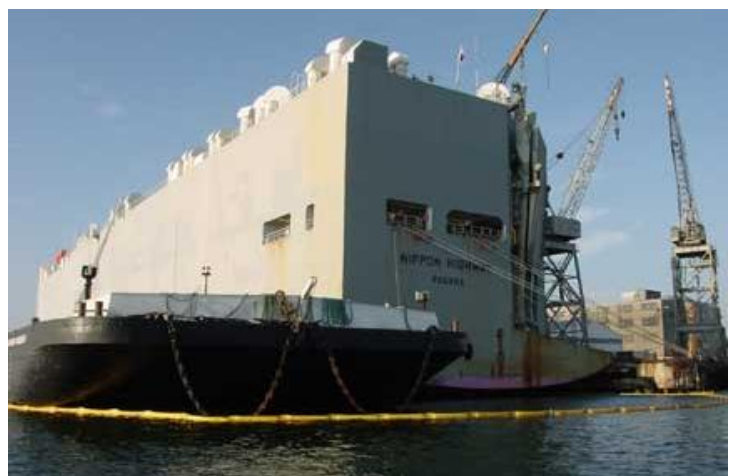
Figure 50. Debunkering 1640 tons from a RORO. Source: [6]
