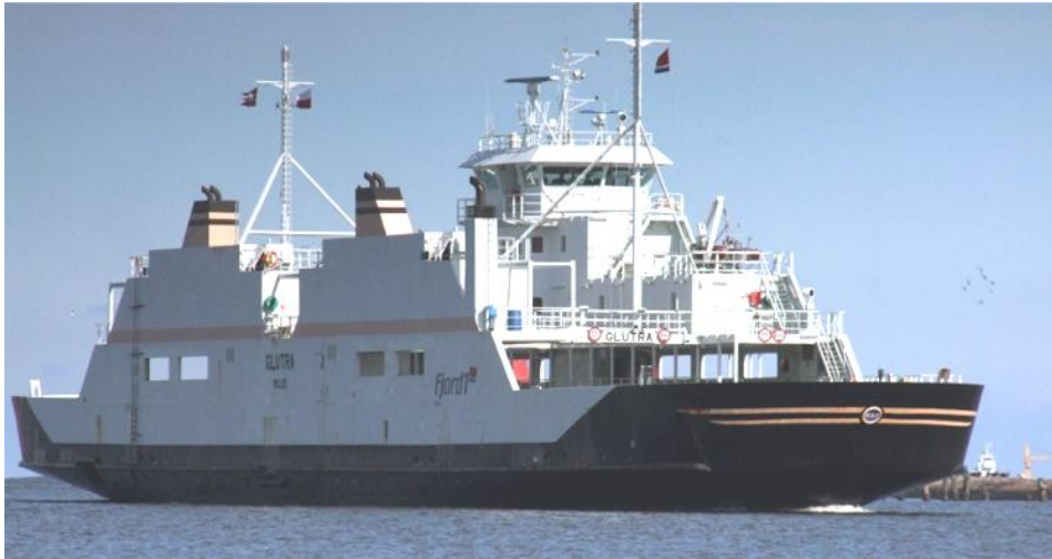
Figure 28. “MF Glutra”. Notice the two separate machine rooms located on the top deck. Picture: vesseltracker.com
