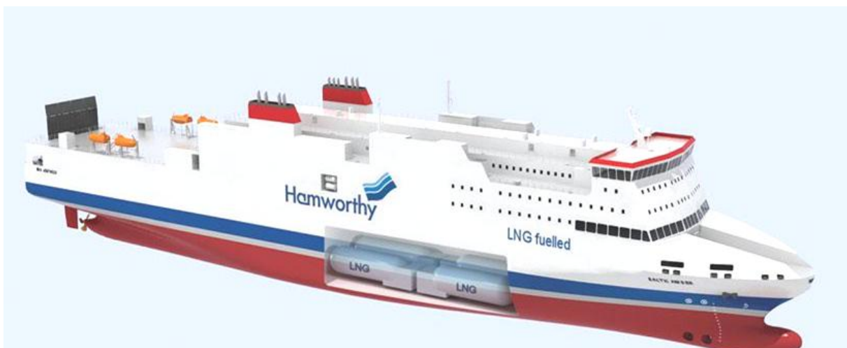
Figure 31. Dual fuel RoPax design from Hamworthy.
