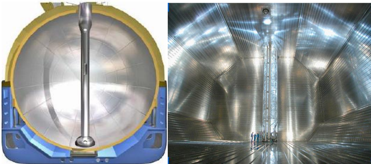
Figure 39. Illustration of a Moss type spherical tank (left), and picture inside of a membrane type tank. (right). Illustrations: [64] and [65]
