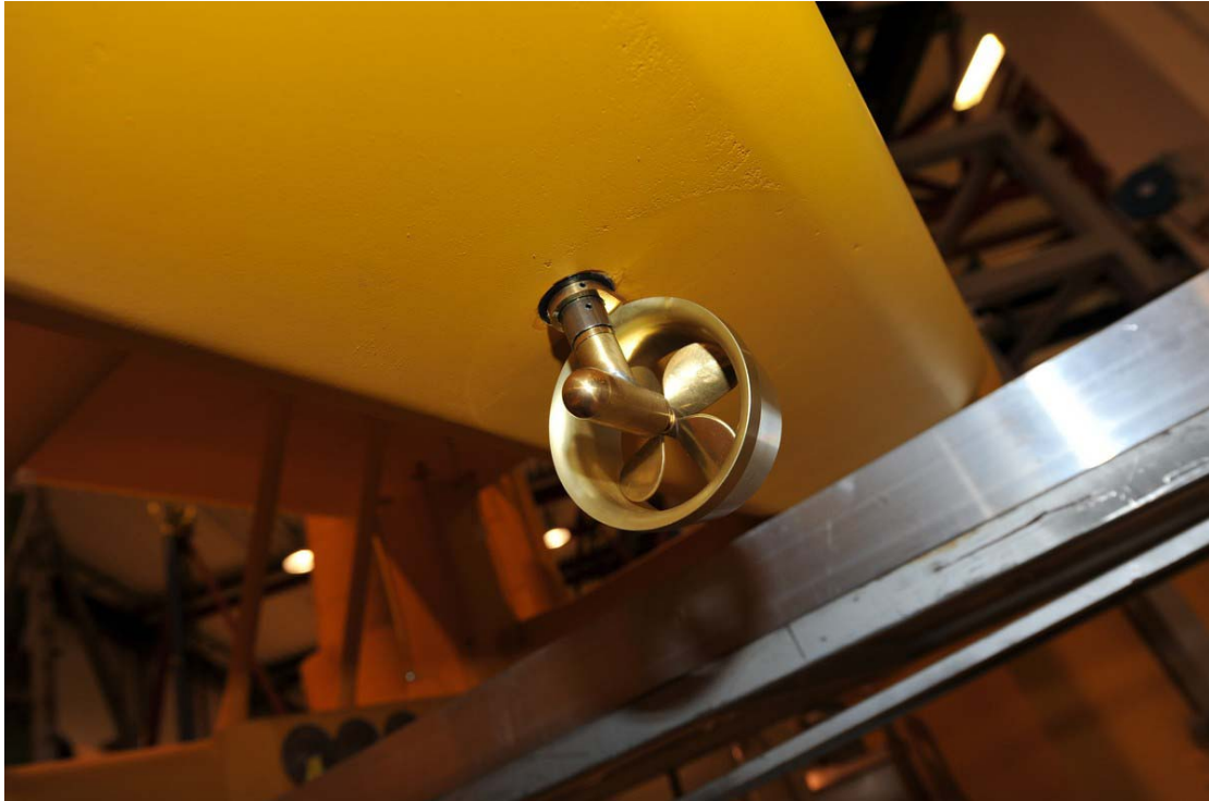
Figure 3.7 Model Thruster as mounted on the model.[6]
