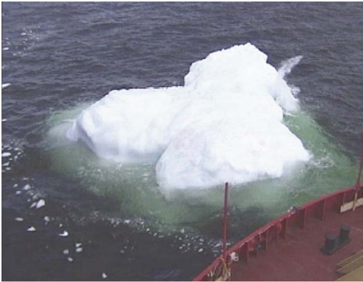
Figure 1-5 Bergy bit impact trials, from Ritch et al. (2008)
