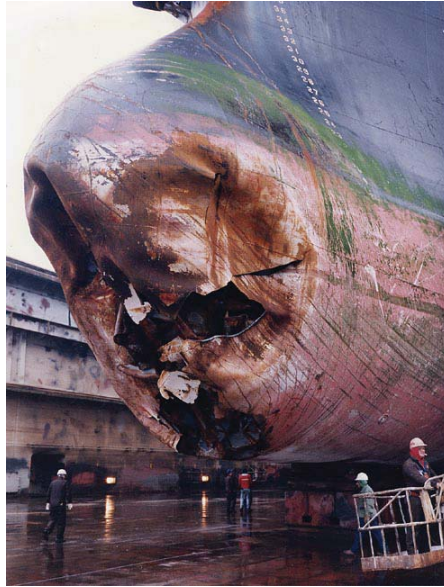
Figure 1-3 Damaged bow of Overseas Ohio after collision with iceberg, from Hill (2006).
