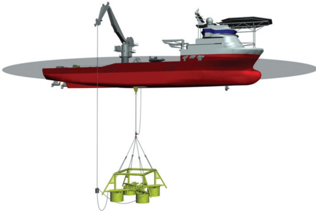
Figure 11 Configuration for installing the template. Reference [4].
