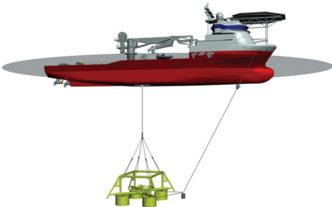
Figure 10 Configuration for transit to deeper waters. Reference [4]
