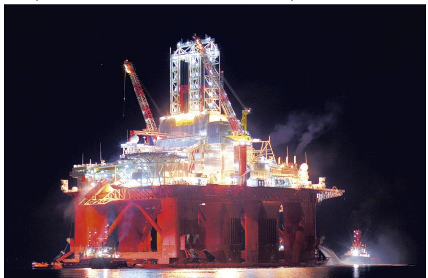
Figure 2 Aker H6 e 6th generation semisub. Note 4 columns on each pontoon, partially submerged. [Maritimt Magasin 2009]
