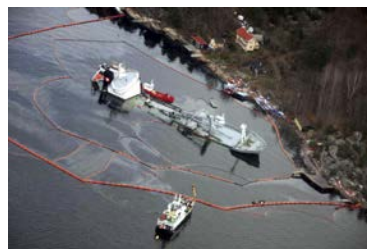
Figure 1.1.4: The “Crete Cement” purposely beached after grounding and taking in water both fore and aft. Photo from the the Accident Investigation Board of Norways official report (Accident Investigation Board Norway and The Bahamas Maritime Authority, 2010).
