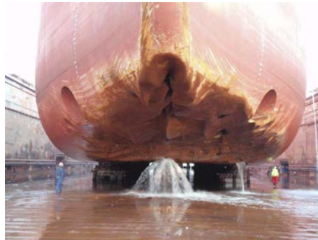
(c) Extensive damage to the bow of the “Federal Kavalina” is seen after the vessel entered dry-dock for repairs
