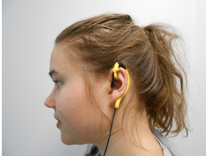
Figure 3.2: Mounting of an ear microphone demonstrated, the shown model is the Sennheiser MKE2 P-C.
