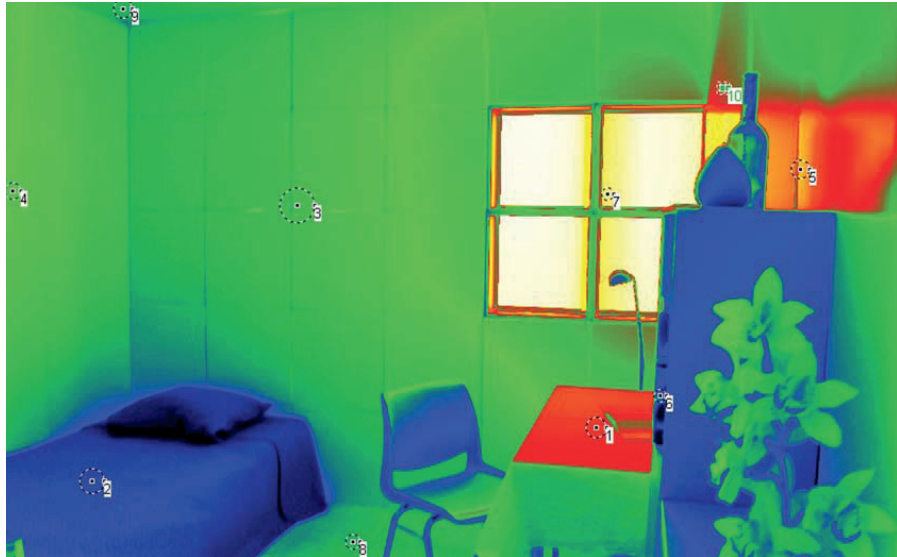
Figure 4: Example - Luminance picture of the RE - White Room, D1. The different colours indicate the approximate value of luminance expressed in cd/m^2 . See graphic bar to the right.
