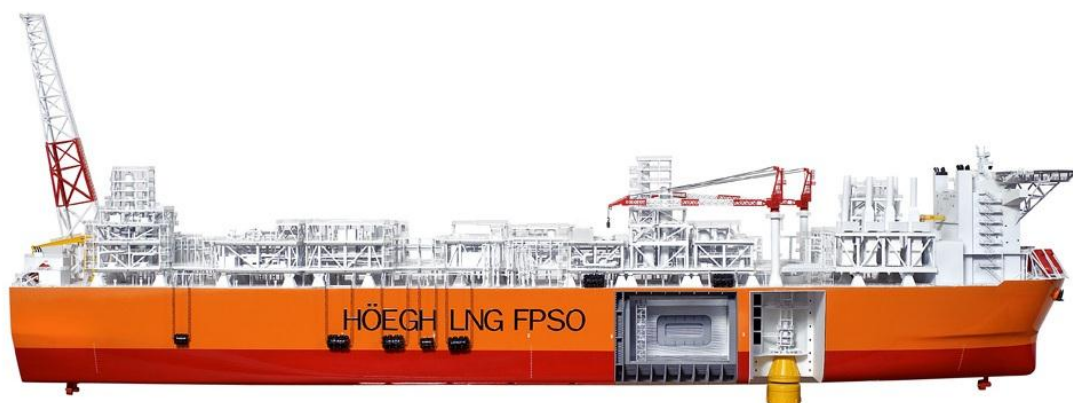
Figure 5-2 View of the dis-connectable turret and of a LNG membrane tank. Source: hoeghlng.com
