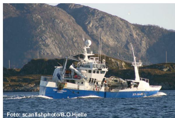
Figure 1.5: Trønderhav before it was rebuilt. We see that it has considerable forward trim in loaded condition. We also see the freeing ports in the net bin at port quarter.
