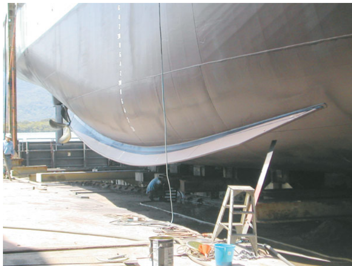
Figure 2.9: A typical bilge keel. The picture is taken from (Australian Government, 2011).
