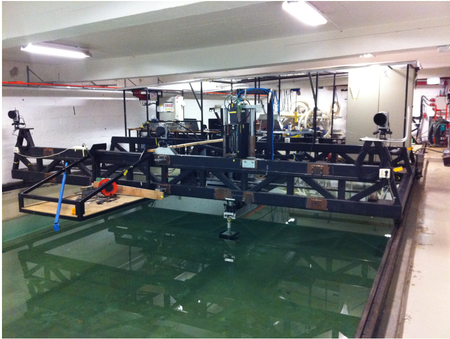
Figure 6: Some of the equipment for the forced oscillation test
