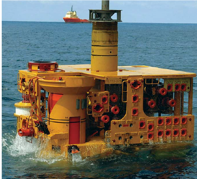
Figure 1: A real life lowering through the wave zone of a XT
