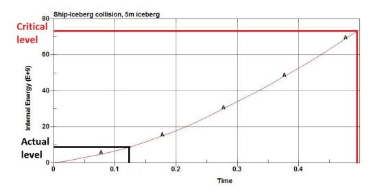
Figure 44: Internal energy plot from LS-DYNA, compared with levels found from 3D external mechanics
