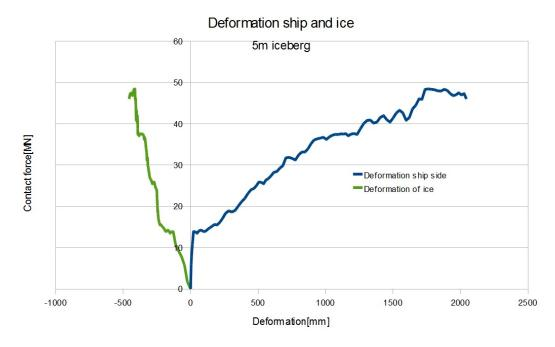
Figure 32: Force vs deformation ship and iceberg
