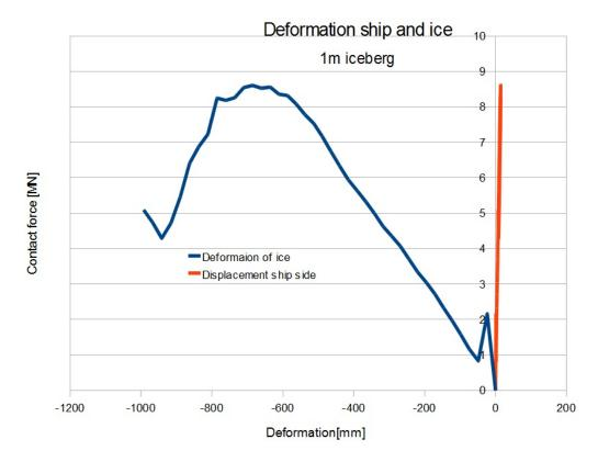
Figure 29: Force vs deformation ship and iceberg
