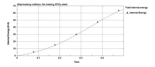
Figure 62: Internal energy 5m iceberg, RTCL-steel
