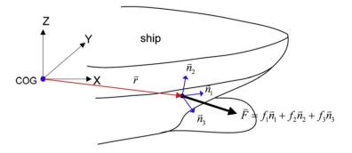
Figure 8: Collision point geometry and local coordinate system, [5]
