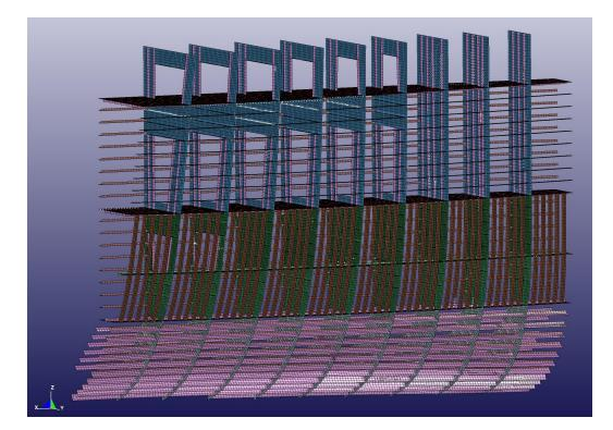
Figure 13: Finished model in LS-PrePost, plating is removed
