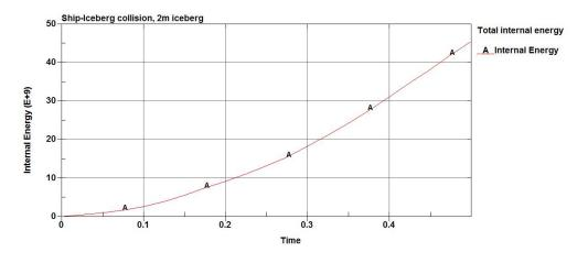
Figure 24: 2m iceberg, Total internal energy in ship and ice
