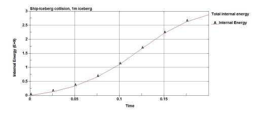
Figure 28: 1m iceberg, Total internal energy in ship and ice
