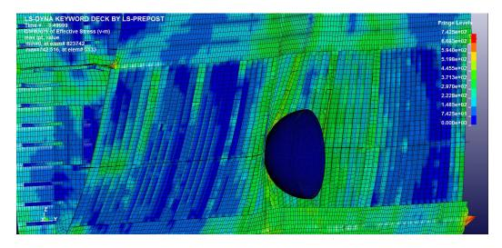
Figure 19: Collision with rigid iceberg, 0.5s, von Mises stress
