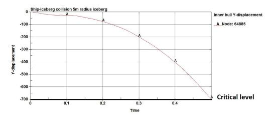
Figure 33: 5m iceberg, Displacement of centre of inner hull
