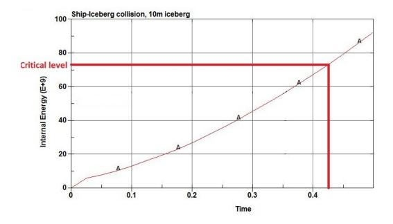
Figure 36: 10m iceberg, Total internal energy in ship and ice
