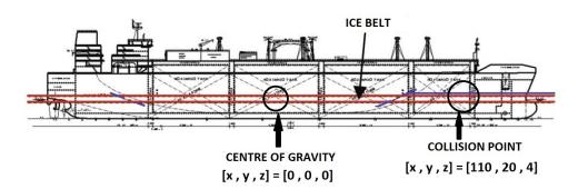
Figure 42: Profile view of 4-tank membrane LNGC
