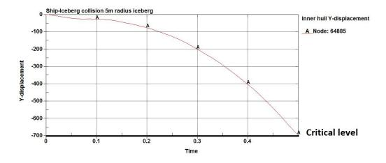
Figure 40: Displacement of the inner hull, central position
