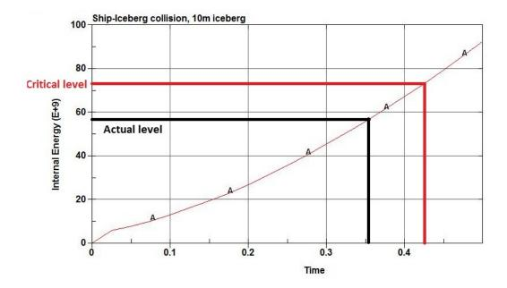
Figure 45: Internal energy plot from LS-DYNA, compared with levels found from 3D external mechanics
