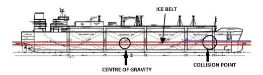
Figure 1: Collision point,[1]
