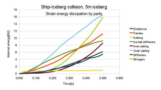
Figure 41: Internal energy by parts
