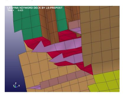
Figure 37: Erosion of elements at the boundaries of the stringers
