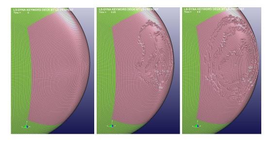
Figure 30: 5m iceberg, stages of collision: 0s, 0.25s, 0.5s
