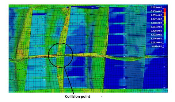
Figure 22: 2m collision, 0.5s, von Mises stress
