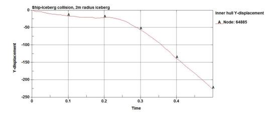
Figure 23: 2m iceberg, Displacement of centre of inner hull
