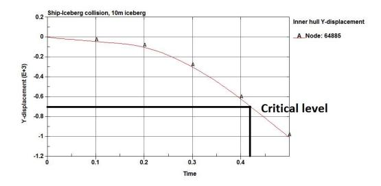
Figure 35: 10m iceberg, Displacement of centre of inner hull
