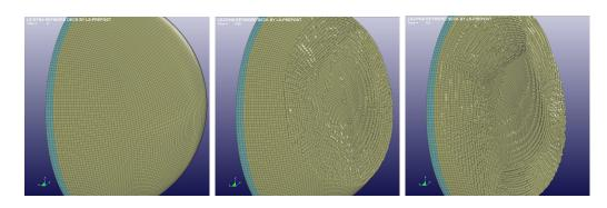
Figure 21: 2m iceberg, stages of collision: 0s, 0.25s, 0.5s
