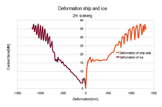
Figure 25: Force vs deformation ship and iceberg
