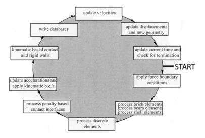
Figure 10: The time integration loop in LS-DYNA, [7]
