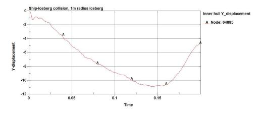
Figure 27: 1m iceberg, Displacement of centre of inner hull
