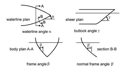
Figure 9: Hull angles, [6]
