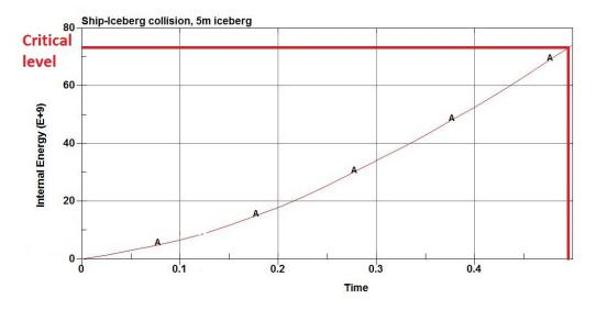
Figure 34: 5m iceberg, Total internal energy in ship and ice
