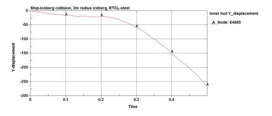
Figure 54: Y-displacement 2m iceberg, RTCL-steel
