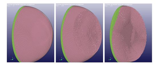
Figure 26: 1m iceberg, stages of collision: 0s, 0.075s, 0.15s
