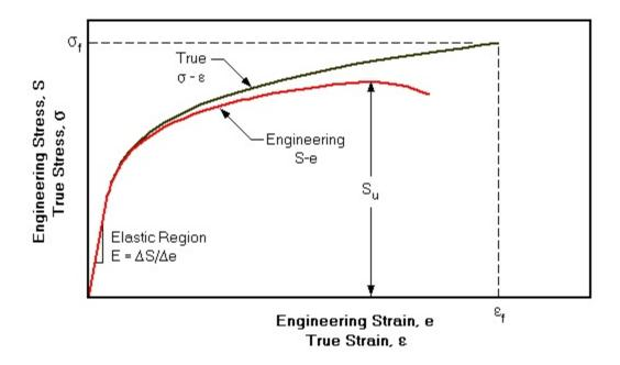
Figure 3: Engineering vs true stress-strain curve
