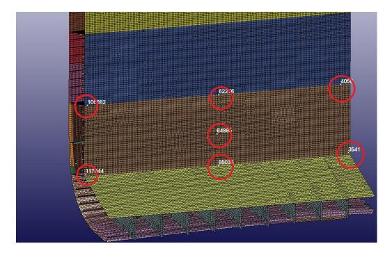
Figure 38: Locations for acceleration check
