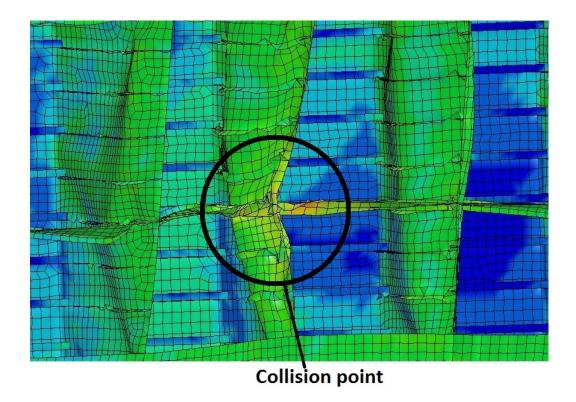
Figure 20: Buckling of frames, 0.5s, von Mises stress
