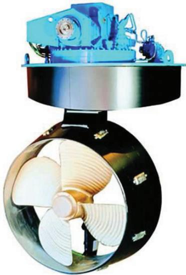
(a) Ulstein Aquamaster azimuth thruster.
