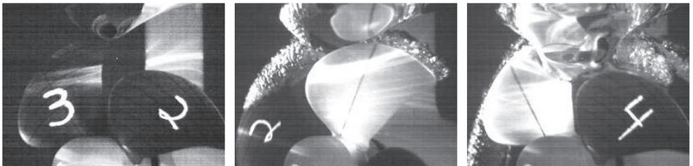
(a) First impact of the propeller on the free-surface,  $t = -0.1388 \text{ s}$ . (b) First impact of  $Blade_1$  on the free-surface,  $t = -0.0972 \text{ s}$ . (c) Minimum blade thrust,  $t = -0.0805 \text{ s}$ .
