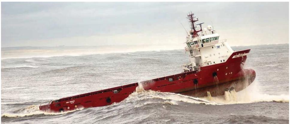
Figure 1.1: Supply vessel operating in heavy sea, where the emersion of the tunnel thrusters on the bow can be observed. Courtesy of Rolls-Royce Marine (RRM).
