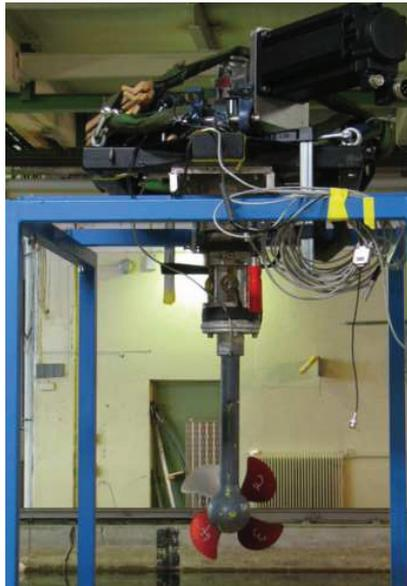
(e) Thruster assembly prior to mounting on the carriage.
