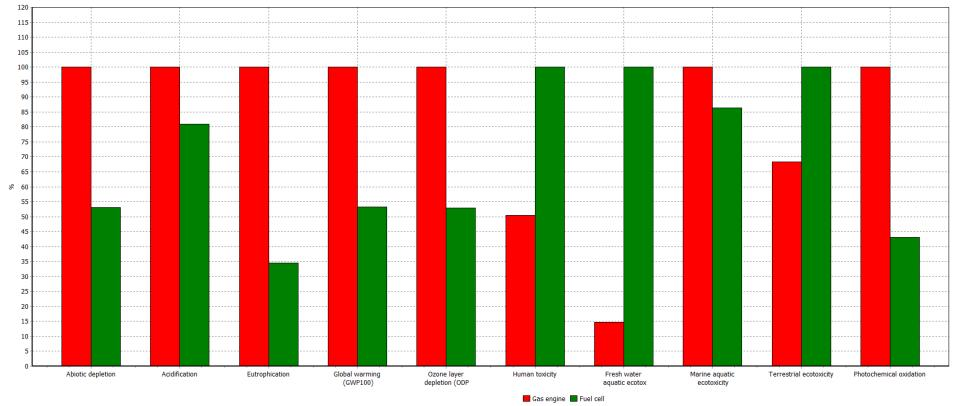
Comparing 1 p 'Gas engine' with 1 p 'Fuel cell'; Method: CML 2 baseline 2000 V2.04 / World, 1990 / characterization
