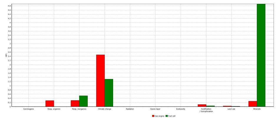
Comparing 1 p 'Gas engine' with 1 p 'Fuel cell'; Method: Eco-indicator 99 (I) V2.04 / Europe EI 99 I/I / weighting
