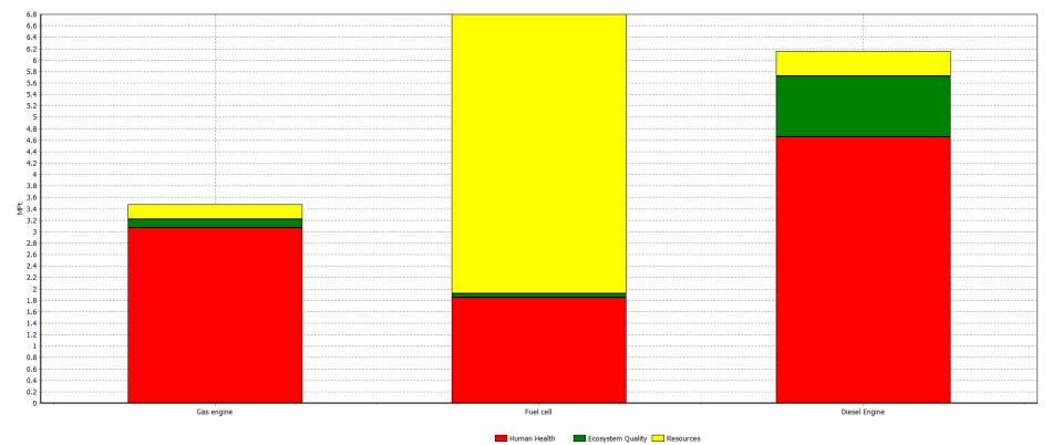
Comparing 1 p 'Gas engine', 1 p 'Fuel cell' and 1 p 'Diesel Engine'; Method: Eco-indicator 99 (I) V2.04 / Europe EI 99 I/I / single score
