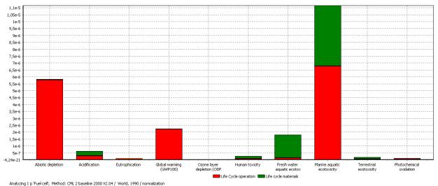
FIGURE 19: TOTAL RESULT FUEL CELL, CML NORMALIZED
