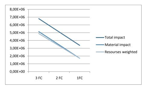
FIGURE 47: IMPACT REDUCTION BY INCREASING FUEL CELL LIFETIME
