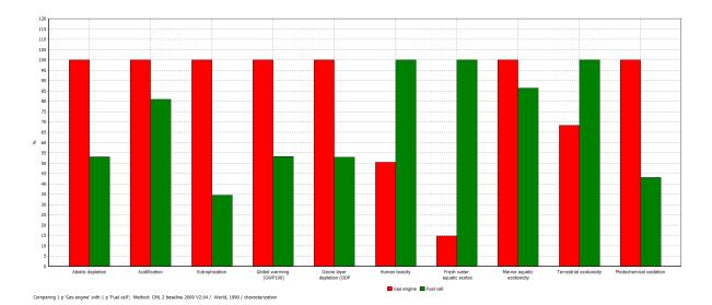
FIGURE 31: GAS ENGINE COMPARED TO FUEL CELL, TOTAL, CML CHARACTERIZED
