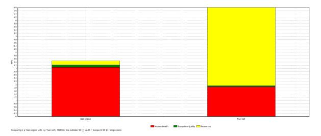
FIGURE 42: GAS ENGINE COMPARED TO FUEL CELL, ECO-INDICATOR SINGLE SCORE
