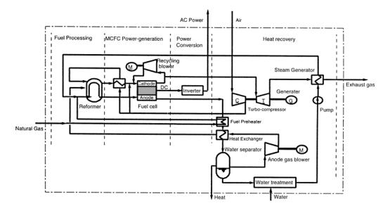
FIGURE 7: MCFC FLOW DIAGRAM (HE 1998)
