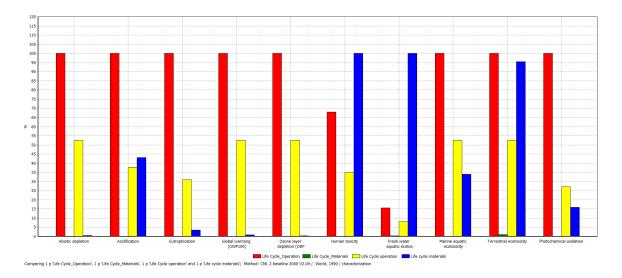
FIGURE 33: GAS ENGINE COMPARED TO FUEL CELL, MATERIAL AND OPERATION, CML CHARACTERIZED
