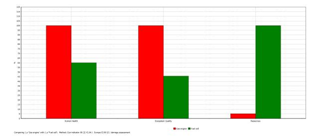
FIGURE 36: GAS ENGINE COMPARED TO FUEL CELL, ECO-INDICATOR DAMAGE ASSESSMENT
