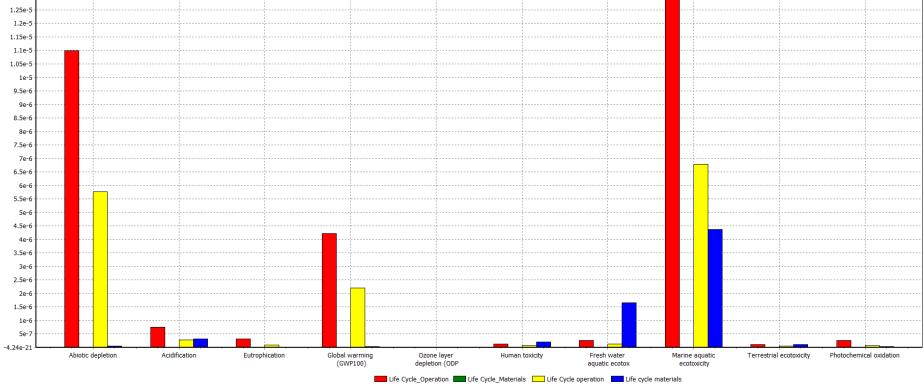
Comparing 1 p 'Life Cycle\_Operation', 1 p 'Life Cycle\_Materials', 1 p 'Life Cycle operation' and 1 p 'Life cycle materials'; Method: CML 2 baseline 2000 V2.04 / World, 1990 / normalization
