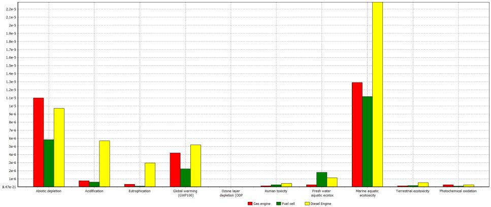
Comparing 1 p 'Gas engine', 1 p 'Fuel cell' and 1 p 'Diesel Engine'; Method: CML 2 baseline 2000 V2.04 / World, 1990 / normalization
