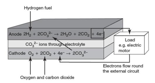
FIGURE 1: FUEL CELL REACTION
