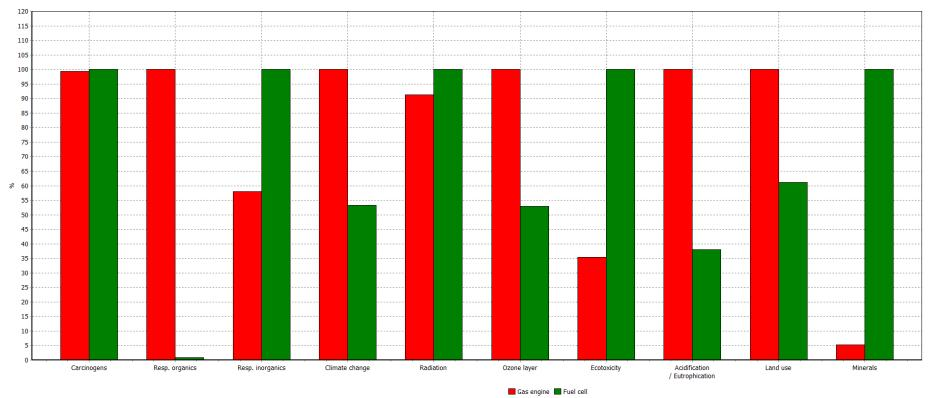
Comparing 1 p 'Gas engine' with 1 p 'Fuel cell'; Method: Eco-indicator 99 (I) V2.04 / Europe EI 99 I/I / damage assessment
