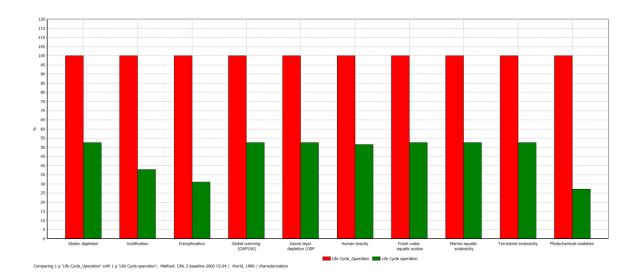
FIGURE 29: GAS ENGINE COMPARED TO FUEL CELL, OPERATION, CML CHARACTERIZED
