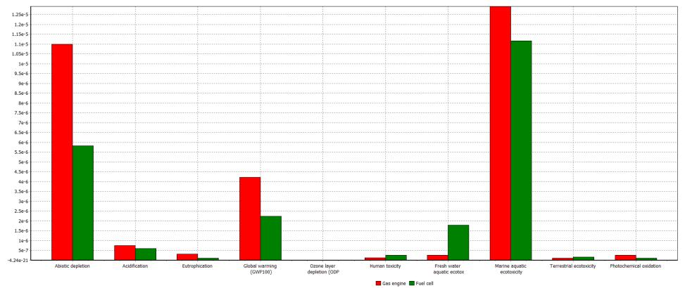
Comparing 1 p 'Gas engine' with 1 p 'Fuel cell'; Method: CML 2 baseline 2000 V2.04 / World, 1990 / normalization
