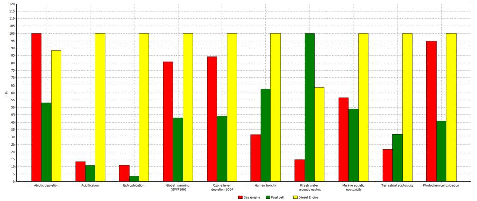
Comparing 1 p 'Gas engine', 1 p 'Fuel cell' and 1 p 'Diesel Engine'; Method: CML 2 baseline 2000 V2.04 / World, 1990 / characterization
