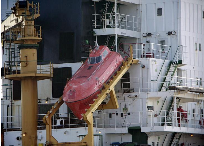
Figure2. A Typical Free-fall Lifeboat
