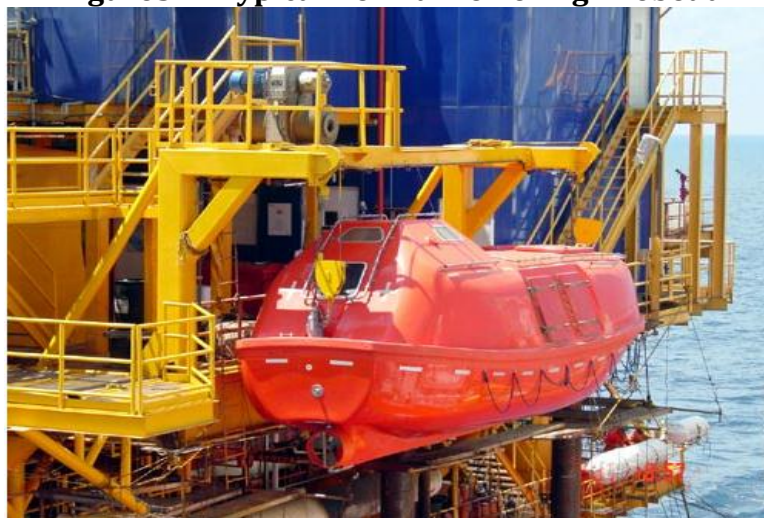
Figure3. A Typical Normal Lowering Lifeboat
