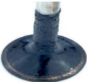
Figure 19: Deposit formation on exhaust valve.
