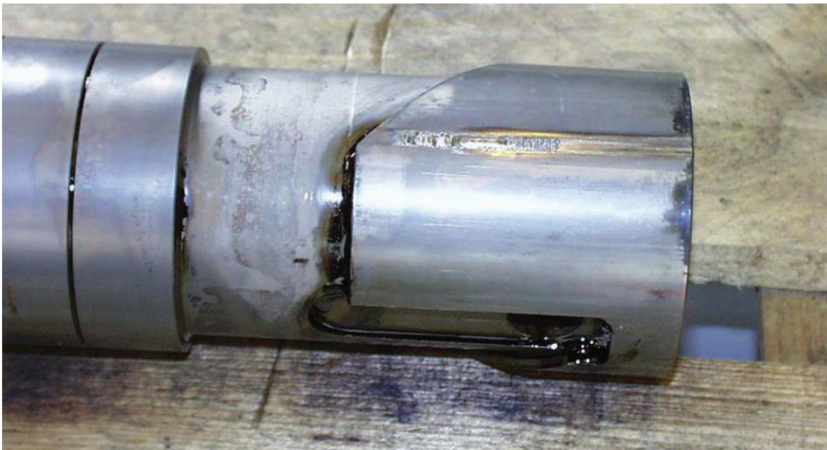
Figure 61: Fuel pump plunger sticking.[31]
