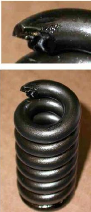
Figure 65: Breakdown of nozzle lifting spring.
